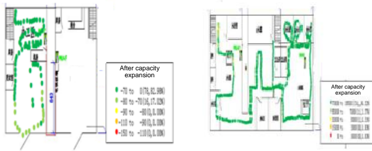
Figure 4-2 Coverage provided by the LampSite solution
