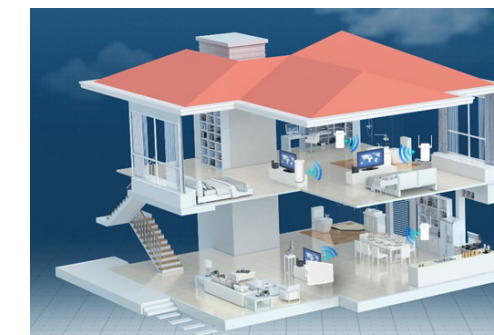
Figure 5-4 Deployment in skip-floor villa scenarios
