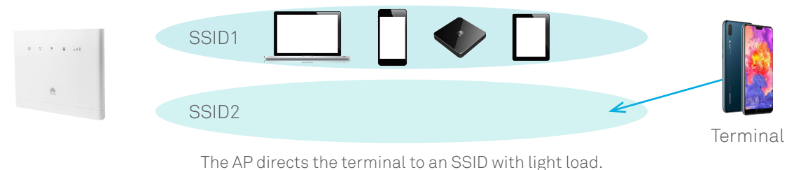
Figure 4-6 Working principle of SSID steering
