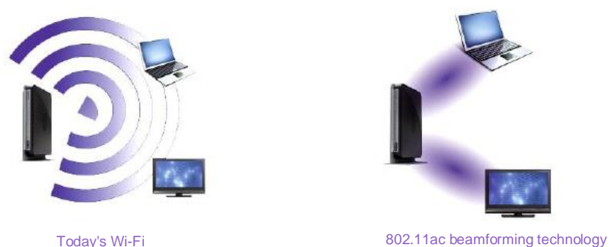
Figure 5-9 Working principle of baseband beamforming
