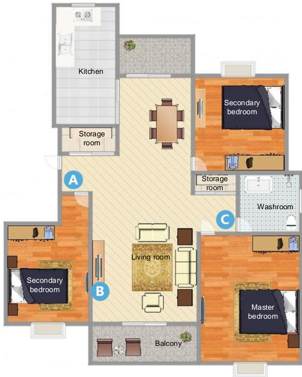
Figure 6-6 Wi-Fi solution design for a house with 3 rooms
