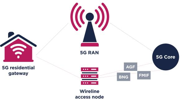
5G RAN = 5G radio access network AGF = Access gateway function, provides AAA services, traffic shaping and policing
