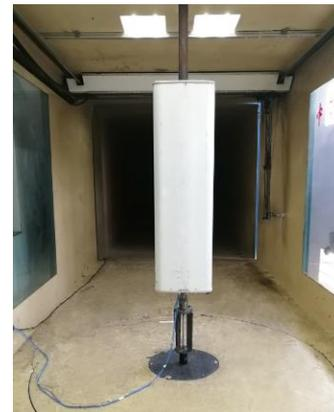
Figure 8 Antenna wind tunnel test in Central South University
