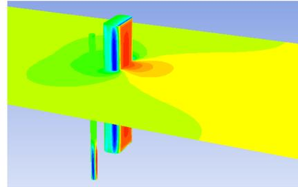
Figure 5 Simulation of antenna wind load
