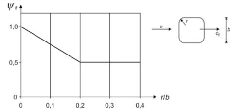
Figure 3 Reduction factor for a rectangular section with rounded corners
