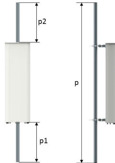
Figure 11 Subtracting the wind load of the pole
