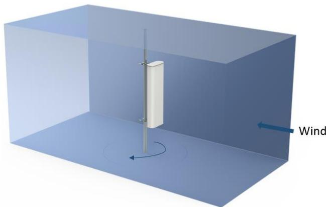
Measure the wind load of the antenna and pole through the wind tunnel test.
