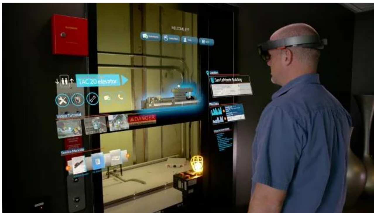
Figure 10: thyssenkrupp technicians using AR for technicians servicing elevators
