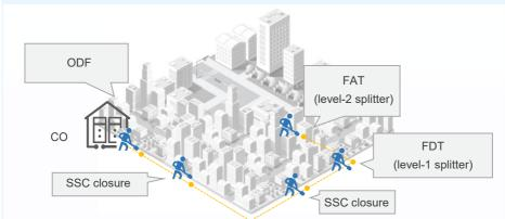
High fiber consumption: More optical cables are needed to enter the building, the rental of the equipment room in the building is high, and optical fibers are difficult to be deployed.
