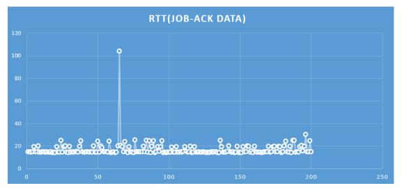
The average RTT is 17 ms. The RTT at one point is large, reaching 104 ms. This value corresponds to the high point of Response Delay in the preceding figure.
