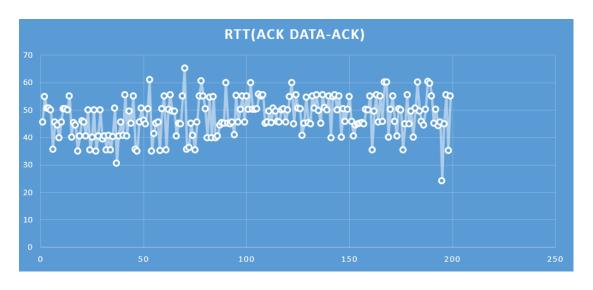
The average latency is 47 ms. Fluctuation is relatively small, ranging from 30 ms to 65 ms; this RTT reflects the network quality from ACK\_DATA to ACK and cannot be covered by Response Delay.
