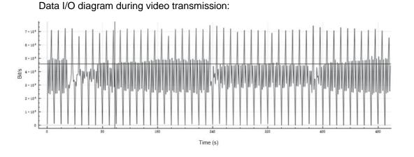
The IP uplink transmission rate is 3 Mbps to 4 Mbps.
