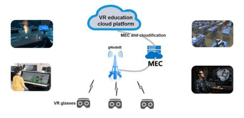
AR/VR teaching contents are uploaded to the cloud. The cloud computing capability is used to implement AR/VR running, rendering, display, and control. The high bandwidth and low latency of 5G are used to transmit the content to VR glasses in real time and construct AR/VR cloud platforms and applications. These include virtual labs, popular science teaching, and 3D interactive classrooms.
