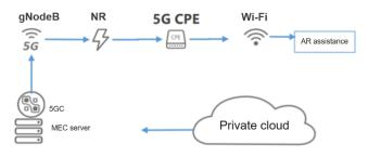
Network requirements: Typical AR glasses are mainly used for 720p video streaming, so 1.5 Mbps downlink rate is required and the latency must be within 20 ms. The 5G + MEC solution is required, as 2K–4K video streams are future demands.
