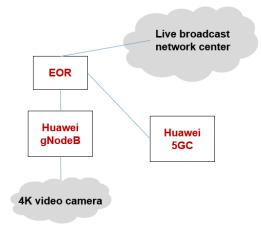
The upload service involves real-time uplink data transmission. The uplink transmission rate is approximately 100 Mbps, which is not necessarily the highest capability of a network. The live broadcast service is transmitted based on the real-time encoding rate of the camera, that is, the average bit rate of 4K videos after real-time encoding is 100 Mbps.
