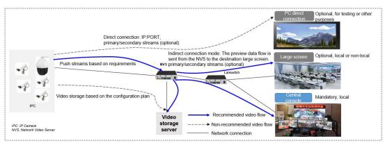
Figure 5-5 Logical networking of the video surveillance service
