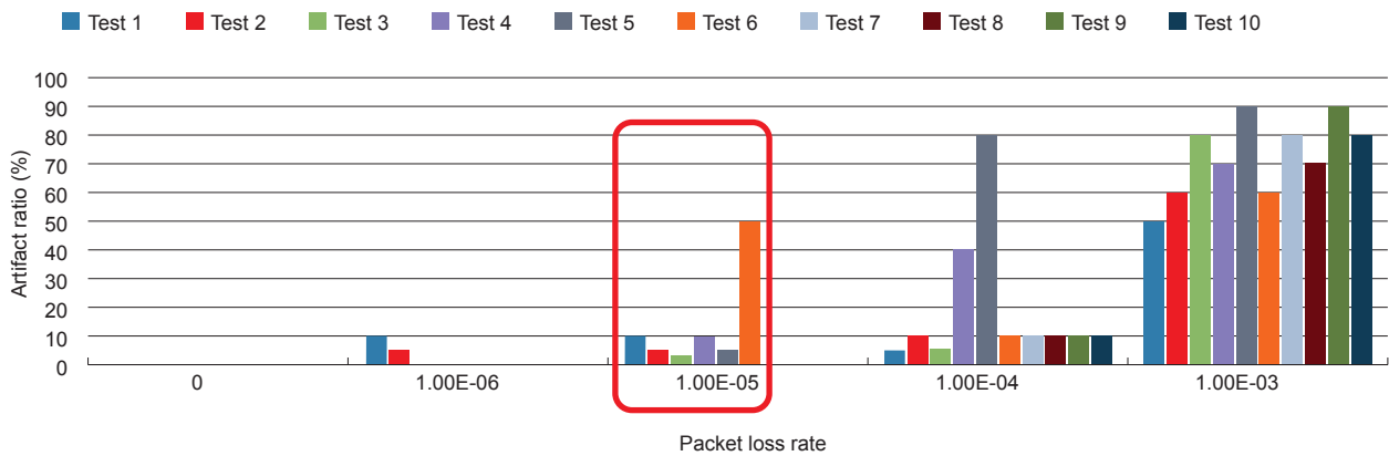
Figure 13: Relationship between the artifact ratio and packet loss rate according to the EDN lab test
