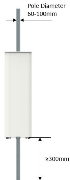
Figure7 Installation spacing requirements of the antenna wind tunnel test
